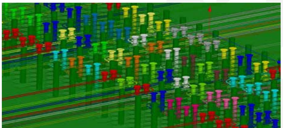
**Figure 4.** Example: signal lines in an ATCA backplane
