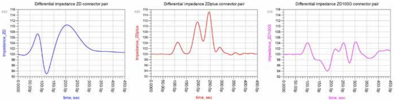
**Figure 3.** Impedance curves in the inserted connector pair (ZD, ZDplus and ZD100G)
