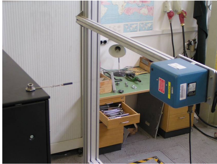
Pic. 6 Measuring equipment LVT for displacement
