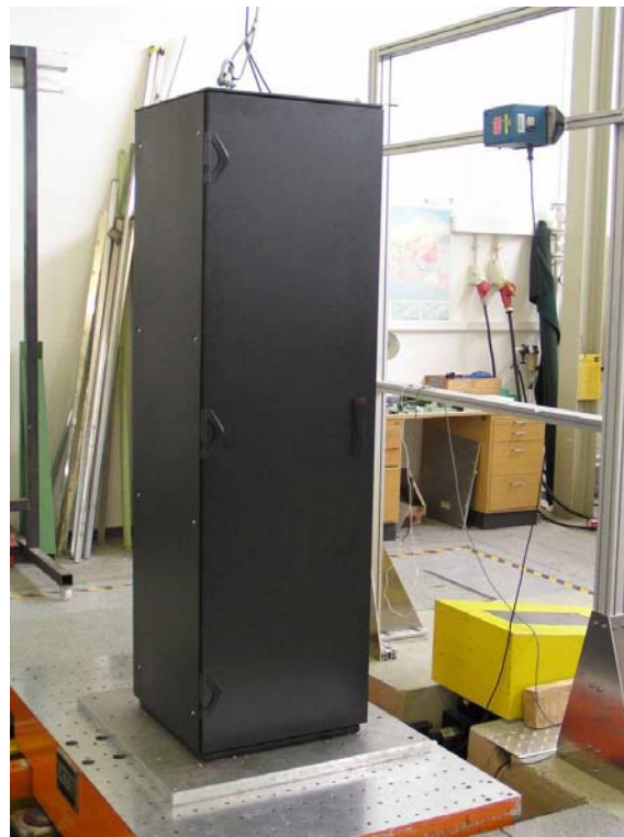
Pic. 7 EUT mounted on the earthquake table
