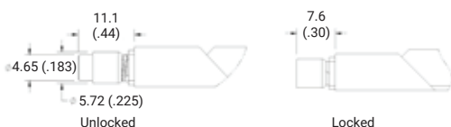
Detail "V" Provides visual lock indication.
