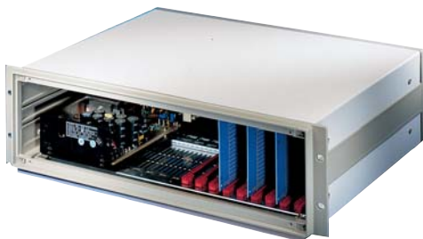
Robust 19" chassis, also for board assembly
