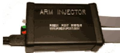
Figure 4.1: Pigeon Point Systems ARM Injector
