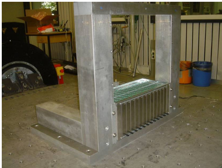
Pic. 4 Mounting of EUT at vibrator table, Y-Axis
