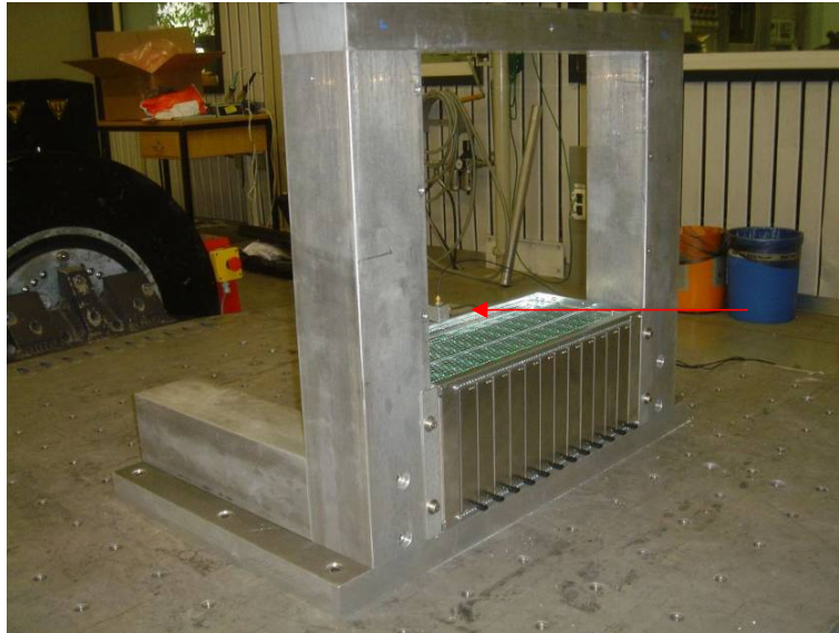
Pic. 5 Position of accelerometers
