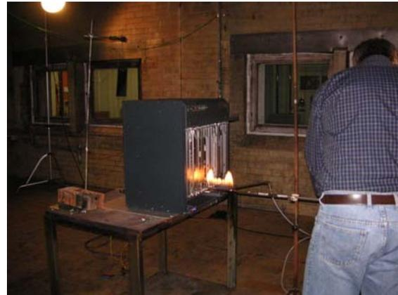
Pic. 13 : Line burner set-up
