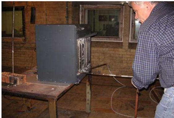
Pic. 10 : Positioning of the line burner
