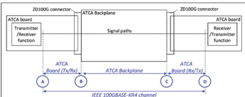
Figure 5. Overview of a 100 Gbps transmission channel
