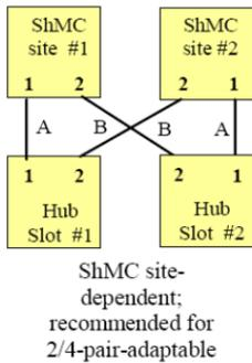
The shelf manager Ethernet ports in a Pentair/Schroff shelf are wired according to the ATCA site-dependent diagram at the left. If only a single switch blade is installed in slot #1, and a shelf manager switchover occurs, shelf manager #2 will not have network connectivity because its port #1 is wired to Hub slot #2 and port #2 is not used in the default configuration.
