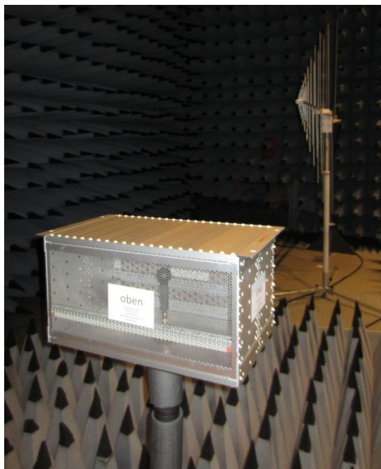
Fig. 5: Setup for the frequency range of 30 MHz - 1 GHz
