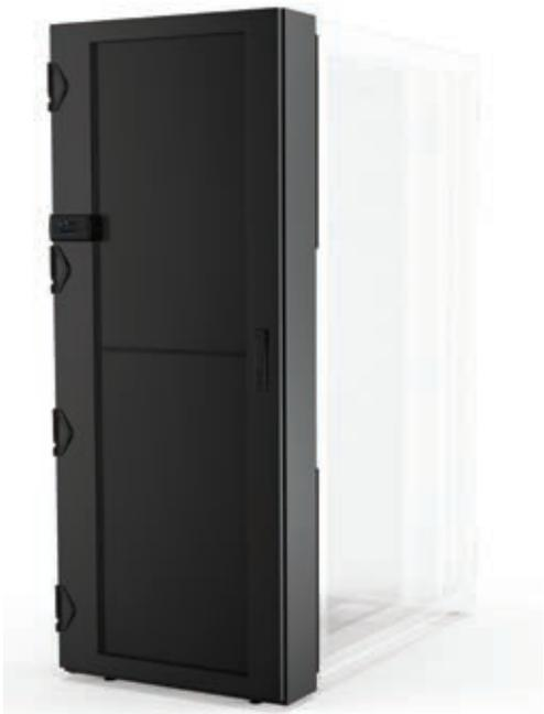
nVent SCHROFF RackChiller Rear Door Chilled Water Heat Exchanger is designed for managing high heat load cooling requirements within higher-density server, computing and storage racks. The entire system is integrated within an aesthetically framed perforated door with protective covers to isolate the liquid source and cooling loop from the rack-mounted equipment. The RDC installs on equipment racks as a separate complete rear door, enabling it to be retrofitted to existing racks.
