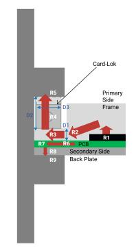
In this VITA 46 example, both a frame and secondary side back plate must be accounted for in the thermal analysis. The hot component is located on the primary side of the frame and the Card-Lok is also mounted on the primary side of the frame.
