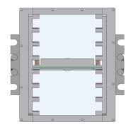
260 Card-Lok mounted to the primary side of the module frame installed in the test fixture
