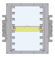
260 Card-Lok mounted to the secondary side of the module frame installed in the test fixture
