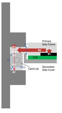
In this VITA 48.2 module configuration, the hot component is located on the primary side of the frame while the Card-Lok is mounted to the secondary side cover.
