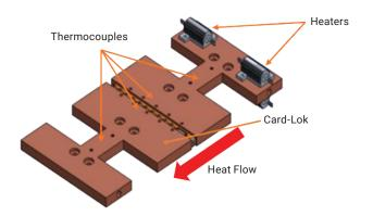
To minimize environmental impacts the fixture is insulated. A chiller is used to cool one end of the fixture to remove residual heat from the system. Below the setup used for testing is depicted, below is the insulated fixture with chillers and not pictured is the test program on the desktop computer that reads the inputs and temperatures throughout the fixture.
