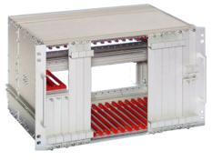
Customer requested a mixed application (3U and 6U boards) assembled into one subrack. The support bars on the side panel, the removable threaded inserts, the Center PIN at the rear side and the option to assembly the flowting connectors was also requested. EM protection was a must.
