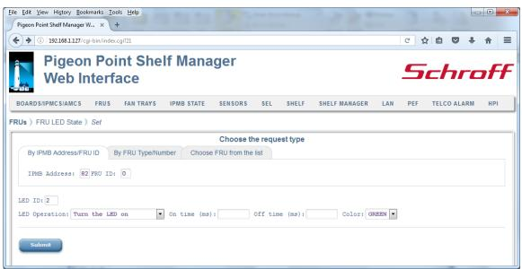
Either the IPMB address of the IPM controller and the FRU device ID or the site type and site number of the target FRU should be specified, or the user can choose the target FRU from a drop-down list of known FRUs in the shelf. The "LED ID" field must be filled with either an LED ID (a numerical value) or ALL. In the latter case, the specified operation applies to all LEDs.
