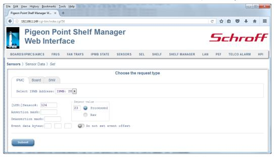
After the user fills in the desired fields and clicks the "Submit" button, the request is executed and a result page is shown, similar to the one below. The output is essentially equal to the output produced by the CLI command setsensordata.
