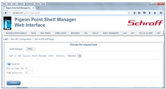
After the user fills in the fields and clicks the "Submit" button, the request is executed and a result page is generated, similar to the one below. The output produced by this command is essentially the same as the output produced by the CLI command setlanconf with the appropriate parameter selector.
