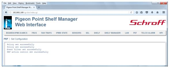
To configure Event Filters, click the "Configure Filters" button. A page, similar to the one below, contains a list of Event Filters and enables the user to inspect and set the Event Filters.
