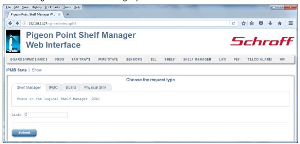
After the user fills in the fields and clicks the "Submit" button, the request is executed and a result page is shown, similar to the one below. The output is essentially equal to the output produced by the CLI command <code>qetipmbstate</code>.
