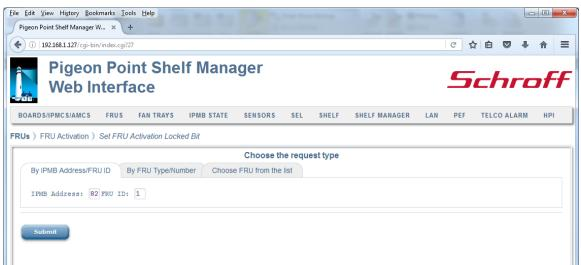
After the user fills in all the fields and clicks the "Submit" button, the request is executed and a result page is produced, similar to the one below. This command is essentially equal to the CLI command setlocked with <value>=1.
