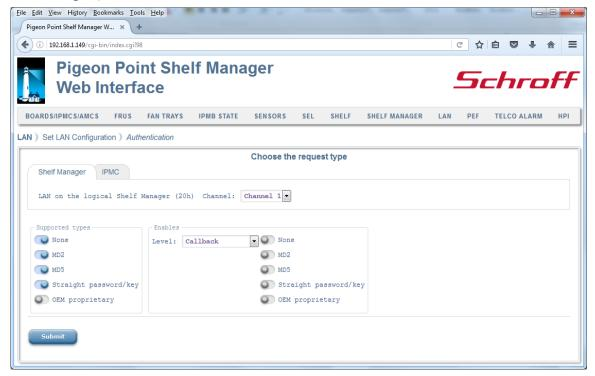
After the user selects the options and clicks the "Submit" button, the request is executed and a result page is generated, similar to the one below. The output produced by this command is essentially the same as the output produced by the CLI command <code>setlanconf</code> with the appropriate parameter selector.
