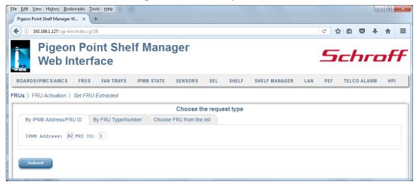
After the user fills in all the fields and clicks the "Submit" button, the request is executed and a result page is produced, similar to the one below. This command is essentially equal to the CLI command setextracted.
