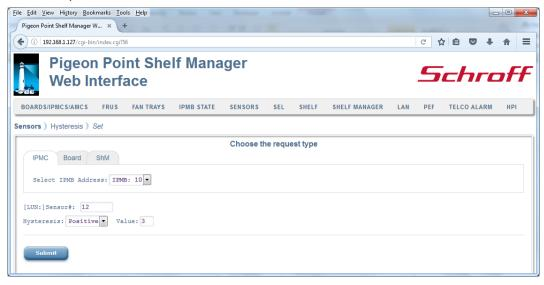
After the user fills in the desired fields and clicks the "Submit" button, the request is executed and a result page is shown, similar to the one below. The output is essentially equal to the output produced by the CLI command <code>sethysteresis</code>.
