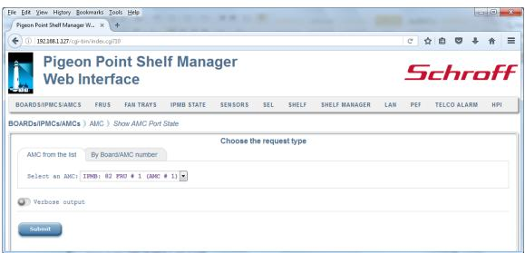
The user chooses the AMC and verbosity of the output and then clicks the "Submit" button. A result page, similar to the one below, appears and shows the state of AMC ports. The AMC can be chosen from a drop-down list or the carrier IPM controller IPMB address and the FRU ID can be specified explicitly.
