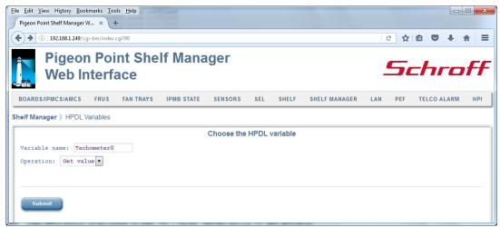
After the user fills in the fields and clicks the "Submit" button, the request is executed and a result page is generated. The output is essentially equal to the output produced by the CLI command variable with appropriate parameters.
