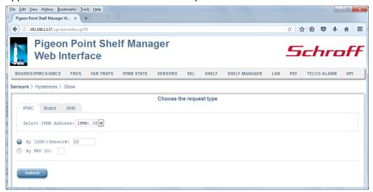
After the user fills in the desired fields and clicks the "Submit" button, the request is executed and a result page is shown, similar to the one below. The output is essentially equal to the output produced by the CLI command gethysteresis.
