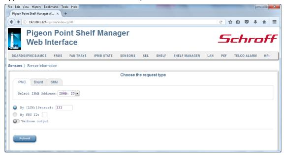
After the user fills in the fields and clicks the "Submit" button, the request is executed and a result page is shown, similar to the one below. The output is essentially equal to the output produced by the CLI command <code>sensor</code>.
