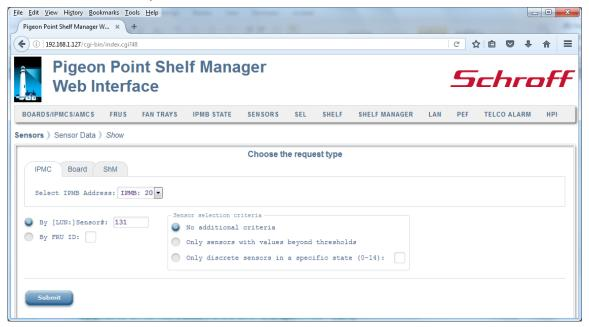
After the user fills in the desired fields and clicks the "Submit" button, the request is executed and a result page is shown, similar to the one below. The output is essentially equal to the output produced by the CLI command sensordata.
