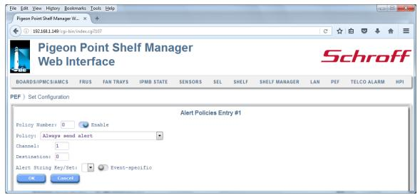
To configure OEM Filters, press the "Configure OEM Filters" button. A page, similar to the one below, displays a list of Active OEM Filters and enables the user to inspect and set the OEM Filters.
