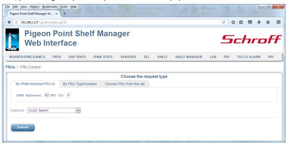
Either the IPMB address of the IPM controller and the FRU device ID or the site type and site number of the target FRU should be specified, or the user can choose the target FRU from the list of known FRUs in the shelf. Also, the user should choose the FRU Control operation.
