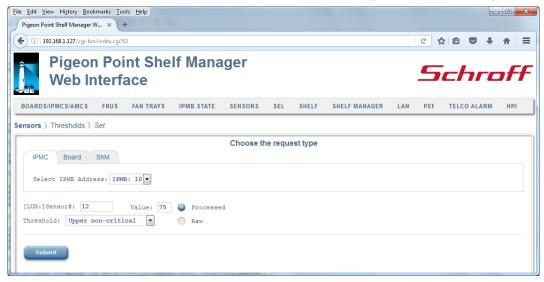
After the user fills in the desired fields and clicks the "Submit" button, the request is executed and a result page is shown, similar to the one below. The output is essentially equal to the output produced by the CLI command setthreshold.
