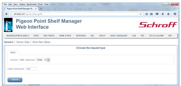
After the user fills in the desired fields and clicks the "Submit" button, the request is executed and a result page is shown, similar to the one below. The output is essentially equal to the output produced by the CLI command sensorread.
