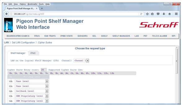
After the user selects options and clicks the "Submit" button, the request is executed and a result page is generated, similar to the one below. The output produced by this command is essentially the same as the output produced by the CLI command setlanconf with the appropriate parameter selector.
