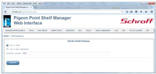
The output is essentially the same as the output produced by the CLI command shelfaddress.
