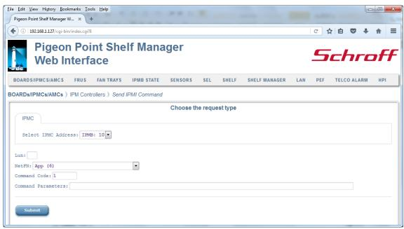
After the user chooses the IPMC address, the LUN (which defaults to 0), NetFn and enters the Command Code and Command Parameters, then clicks the "Submit" button, the request is executed and a result page is shown, similar to the one below. The command code and parameters should be specified as hexadecimal bytes (with the bytes for each parameter separated by spaces). The output is essentially equal to the output produced by the CLI command <code>sendcmd</code>.
