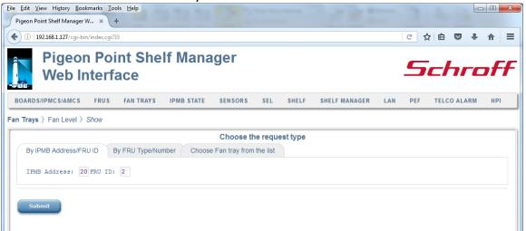
After the user fills in the desired fields and clicks the "Submit" button, the request is executed and a result page is shown, similar to the one below. The output is essentially equal to the output produced by the CLI command <code>qetfanlevel</code>.
