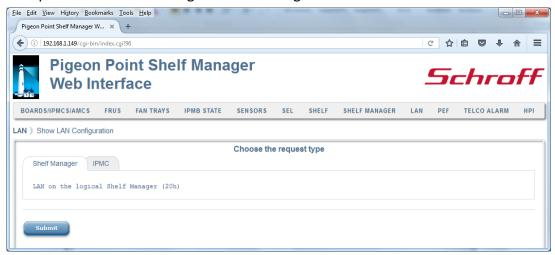
After the user selects the target of the operation and clicks the "Submit" button, the request is executed and a result page is generated, similar to the one below. The output produced by this command is essentially the same as the output produced by the CLI command getlanconf.
