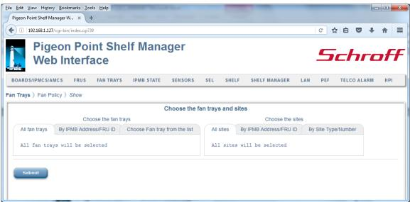
After the user fills in the desired fields and clicks the "Submit" button, the request is executed and a result page is shown, similar to the one below. The output is essentially equal to the output produced by the CLI command <code>getfanpolicy</code>.
