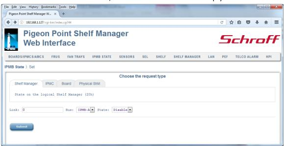
After the user fills in the fields and clicks the "Submit" button, the request is executed and a result page is shown, similar to the one below. The output is essentially equal to the output produced by the CLI command <code>setipmbstate</code>.
