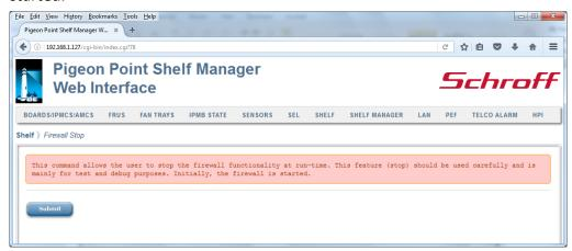
The output is essentially equal to the output produced by the CLI command firewall stop.
