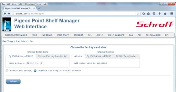
After the user fills in the desired fields and clicks the "Submit" button, the request is executed and a result page is shown, similar to the one below. The output is essentially equal to the output produced by the CLI command setfanpolicy.
