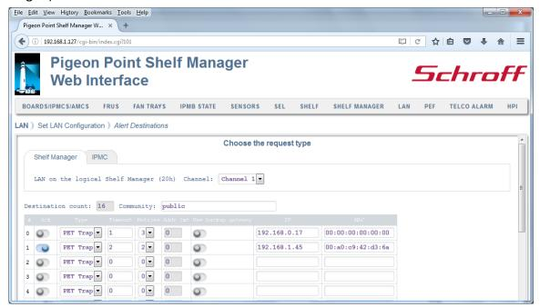
After the user fills in the fields and clicks the "Submit" button, the request is executed and a result page is generated, similar to the one below. The output produced by this command is essentially the same as the output produced by the CLI command setlanconf with the appropriate parameter selector.
