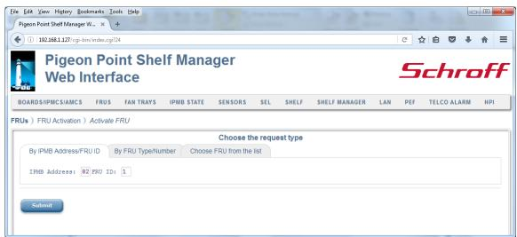
After the user fills in all the fields and clicks the "Submit" button, the request is executed and a result page is produced, similar to the one below. This command is essentially equal to the CLI command activate.
