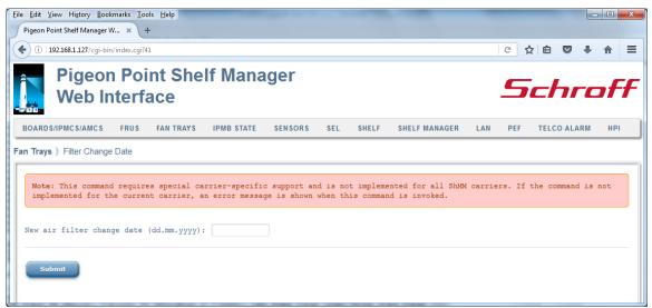
After the user fills in the field and clicks the "Submit" button, the request is executed and a result page is shown, similar to the one below. The output is essentially equal to the output produced by the CLI command <code>airfilterreplaced</code>.
