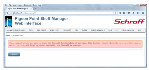
The output is essentially equal to the output produced by the CLI command firewall start.
