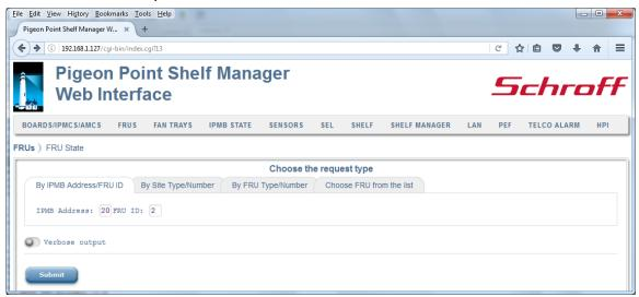
After the user fills in the desired fields and clicks the "Submit" button, the request is executed and a result page is shown, similar to the one below. The output is essentially equal to the output produced by the CLI command fru.
