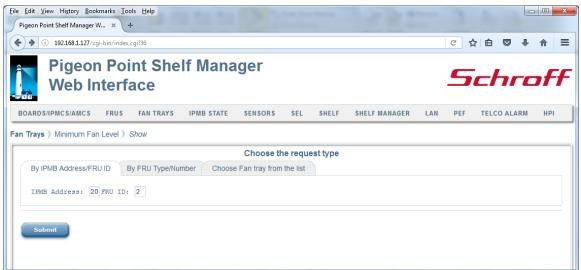
After the user fills in the desired fields and clicks the "Submit" button, the request is executed and a result page is shown, similar to the one below. The output is essentially equal to the output produced by the CLI command minfanlevel in "get" mode.
