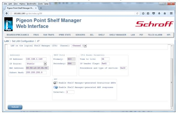
After the user fills in the fields and clicks the "Submit" button, the request is executed and a result page is generated, similar to the one below. The output produced by this command is essentially the same as the output produced by the CLI command setlanconf with the appropriate parameter selector.
