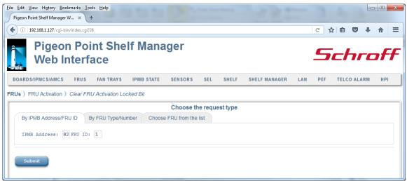
After the user fills in all the fields and clicks the "Submit" button, the request is executed and a result page is produced, similar to the one below. This command is essentially equal to the CLI command setlocked with <value>=0.
