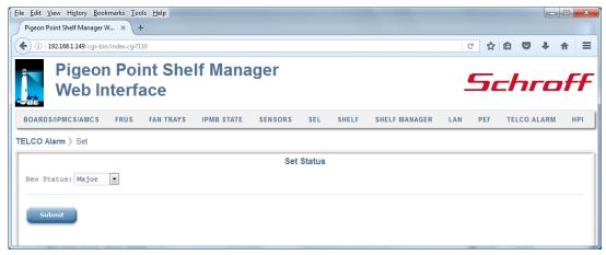
After the user chooses the alarm to set and clicks the "Submit" button, the request is executed and a result page is shown, similar to the one below. It displays the output produced by the CLI commands alarm with a correspondent parameter and alarm info.
