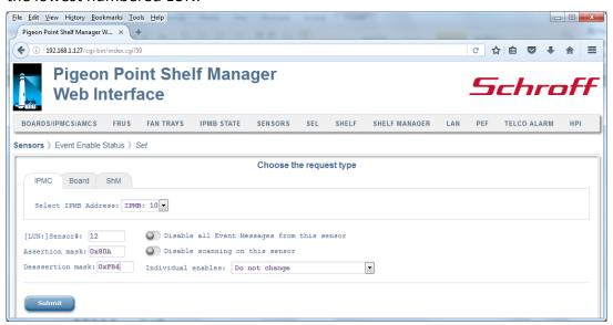
After the user fills in the request information and clicks the "Submit" button, the request is executed and a result page is generated, similar to the one below. The output produced by this command is essentially the same as the output produced by the CLI command setsensoreventenable.
