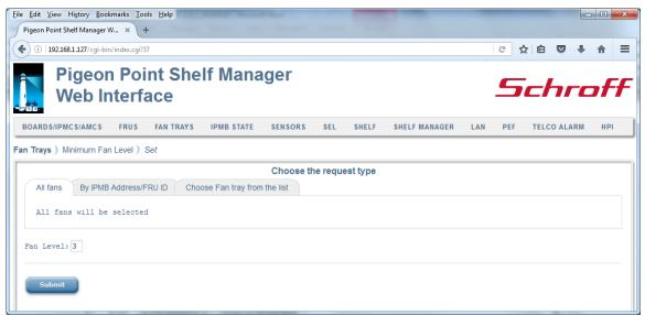
After the user fills in the desired fields and clicks the "Submit" button, the request is executed and a result page is shown, similar to the one below. The output is essentially equal to the output produced by the CLI command minfanlevel in "set" mode.
