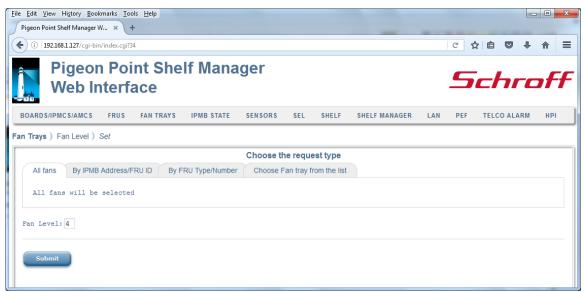
After the user fills in the desired fields and clicks the "Submit" button, the request is executed and a result page is shown, similar to the one below. The output is essentially equal to the output produced by the CLI command setfanlevel.
