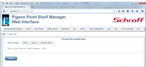
After the user chooses the desired option and clicks the "Submit" button, the request is executed and a result page is shown, similar to the one below. The output is essentially equal to the output produced by the CLI command  $sel\ clear$ .
