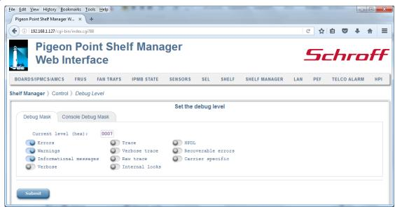
The output is essentially equal to the output produced by the CLI command debuglevel.
