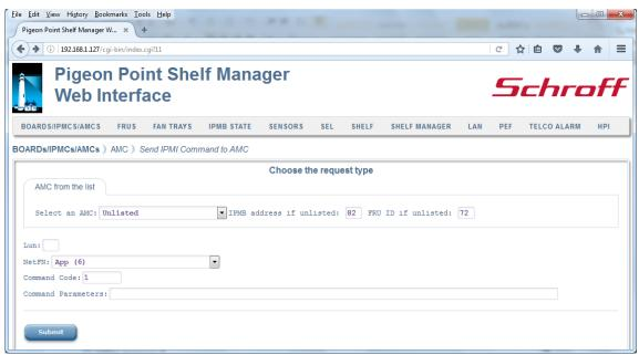
After the user chooses the AMC, NetFn and enters the Command Code and Command Parameters, then clicks the "Submit" button, the request is executed and a result page is shown, similar to the one below. The AMC can be chosen from a drop-down list or the carrier IPM controller IPMB address and the FRU ID can be specified explicitly. The command code and parameters are specified as hexadecimal bytes (with the bytes for each parameter separated by spaces).
