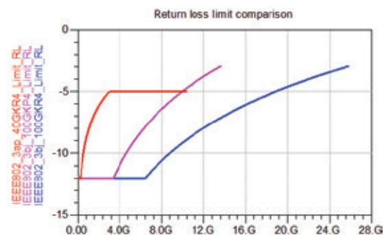
Figure 2. Return loss comparison
