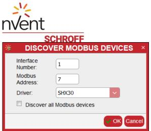
The following drivers for serial Modbus devices are installed by default: "SHX30", "TTSIM", "Omron", "Raychem", "HoffmanCNQDValue", "Yeeka15xx". Other drivers may be added via the "Modbus JSON Drivers" dialog window, which is invoked by the "Maintenance" -> "Modbus" -> "Modbus JSON Drivers" menu item (see section 0).
