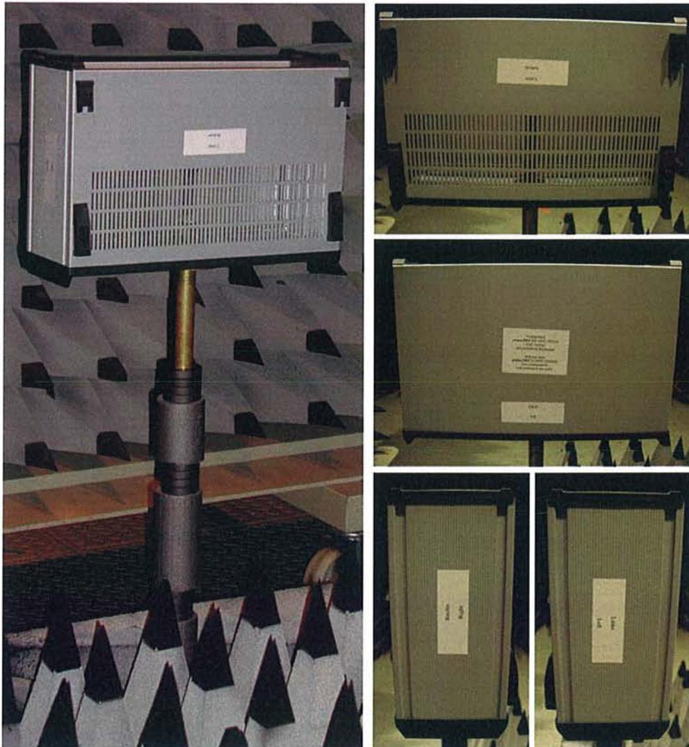
Fig. 1: EUT at the measurement position inside the anechoic chamber
