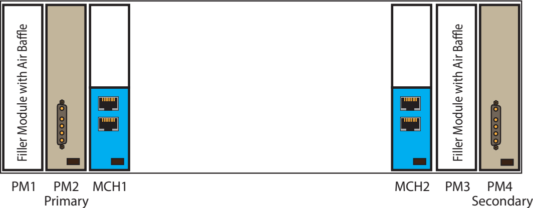
Example 2: 2 x Double 12 HP Power Modules (Supported by factory FRU File)
