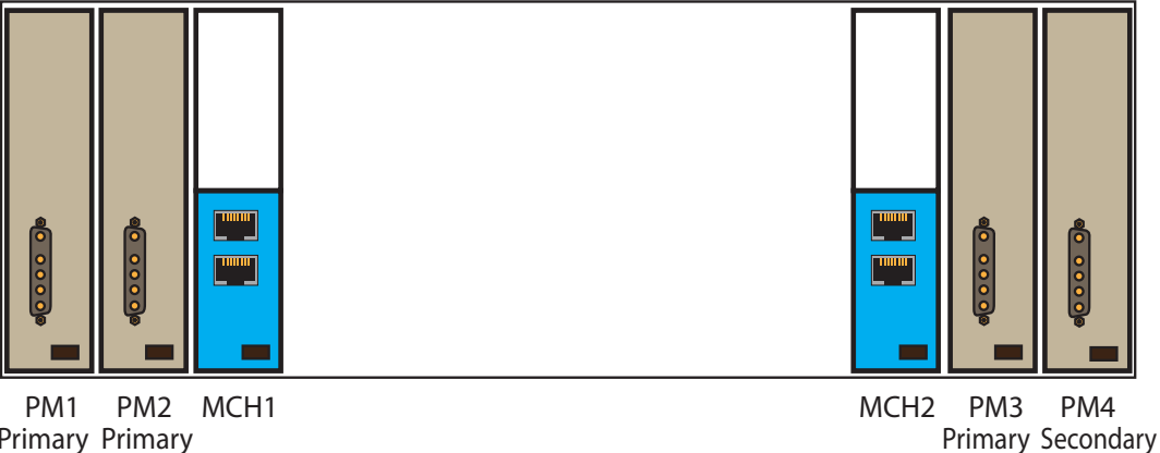
Example 1: 4 x Double Full-size Power Modules (Custom specific FRU File)
