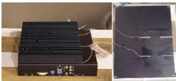
Figure 13: COM carrier in the climate chamber equipped with sensors and a Schroff heat sink (left); position of the temperature sensors glued into the grooves (right).
