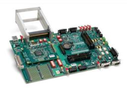
Supported SmartFusion intelligent mixed-signal FPGAs include the A2F200 and A2F500, with CS288, FG256 and FG484 packages. Please refer to Microsemi documentation for details of the differences in capabilities among these devices and see the separate *Pigeon Point BMR-A2F IPMC Product Brief* for more details on the reference design.
