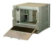
The requirement for high shock and vibration resistance is met due to the use of our robust EuropacPro rugged subrack and meets the requirement for MIL-STD 710F and MIL-STD 167. The EMC shielding requirements according to MIL-STD 461 have been realized by a 2 level shielding concept. The chassis itself and a special shielding of the front and rear card cages define the 2 shielding levels. The system can be integrated into the corresponding MIL cabinets due to the optional front-to-back cooling.
