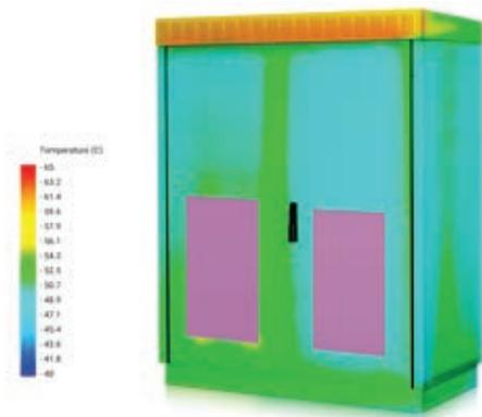
The nVent SCHROFF engineering team used thermal modeling to create a customized cooling solution, ensuring each heat pocket in the outdoor modular cabinet is optimally cooled while balancing the overall energy usage of the cooling system.
