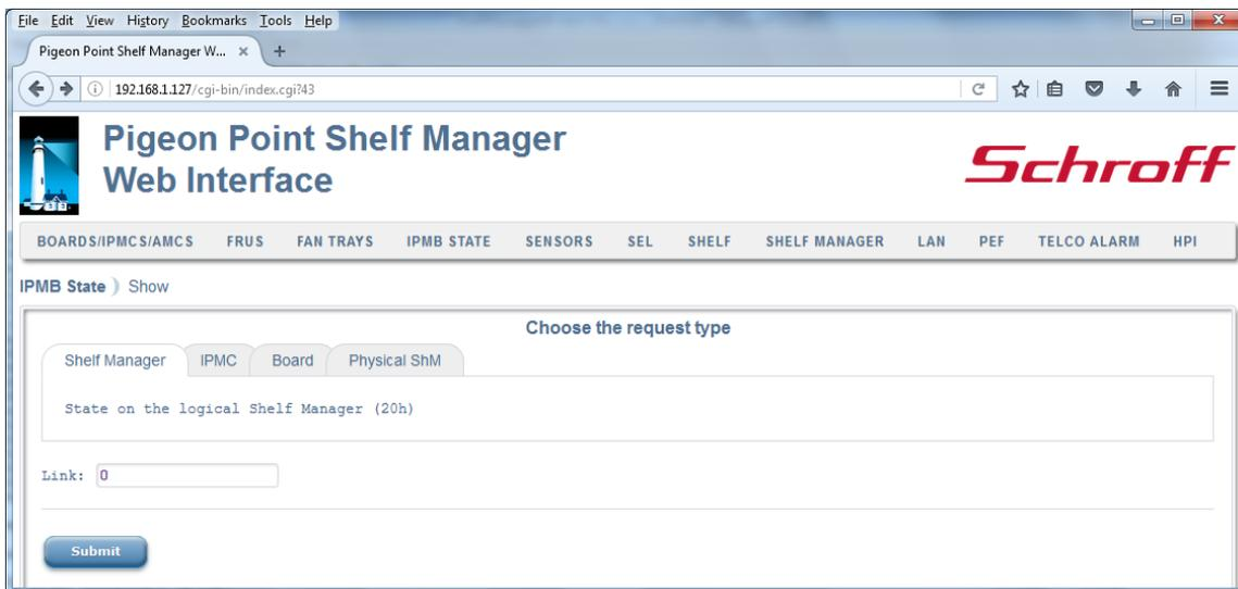
After the user fills in the fields and clicks the “Submit” button, the request is executed and a result page is shown, similar to the one below. The output is essentially equal to the output produced by the CLI command *getipmbstate*.
