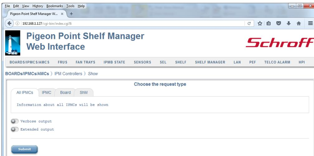
After the user fills in the desired fields and clicks the “Submit” button, the request is executed and a result page is shown, similar to the one below. The output is essentially equal to the output produced by the CLI command *ipmc*.
