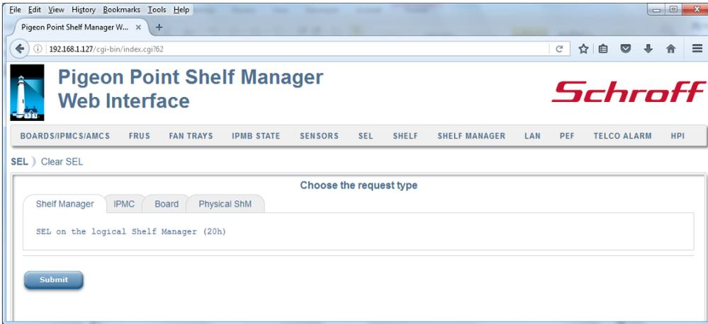
After the user chooses the desired option and clicks the “Submit” button, the request is executed and a result page is shown, similar to the one below. The output is essentially equal to the output produced by the CLI command `sel clear`.
