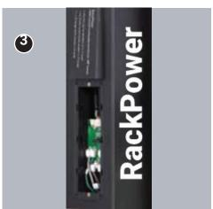
Step 3: Unscrew and pull out the faulty RP meter
