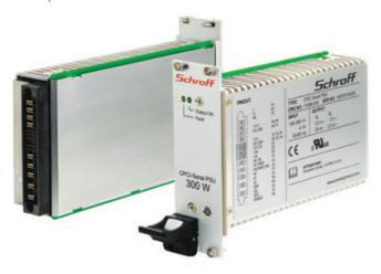
Instead of a pluggable unit the user may prefer an open frame PSU which usually provides a higher output power. With the various configurations nVent is able to cover 98% of all requirements for CPCI Serial applications. The power input is as for CompactPCI at the backside of the unit. This supports a power entry at the rear side of the system which avoids any disruptive cabling at the front.
