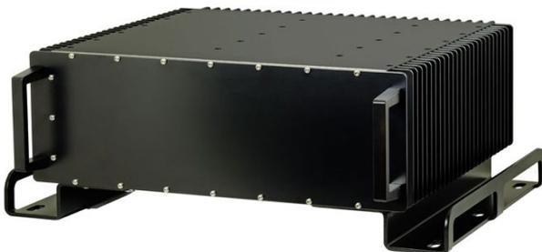
A conduction cooled chassis for this application was mandatory. A Flotherm simulation was performed to analyze and optimize the thermal solution. Special clamshells were developed to get a sufficient heat transfer from the inserted boards to the chassis. The backplane design was made according to customers' requirements.
