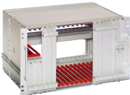
Customer requested a mixed application (3U and 6U boards) assembled into one subrack. The support bars on the side panel, the removable threaded inserts, the Center PIN at the rear side and the option to assembly the floating connectors was also requested. EM protection was a must.
