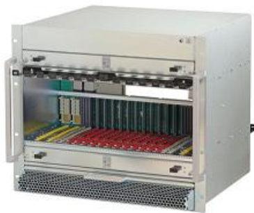
Fig.: Schroff Standard MicroTCA.4 system, 9 U, 12 Slots
