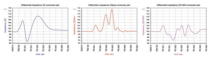
Figure 3. Impedance curves in the inserted connector pair (ZD, ZDplus and ZD100G)
