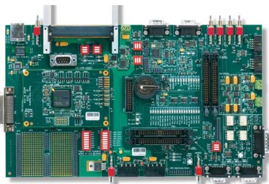
Supported SmartFusion intelligent mixed-signal FPGAs include the A2F200 and A2F500, with CS288, FG256 and FG484 packages. Please refer to Microsemi documentation for details of the differences in capabilities among these devices and see the separate *Pigeon Point BMR-A2F-VPX Product Brief* for more details on the reference design.
