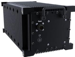
Rugged MicroTCA, MTCA.3, was chosen as it gives the needed robustness and computing power. The cooling performance was optimized by simulations and measurements. A special power supply board was developed to fit into the dimensions of the box and generate enough power for the application.
