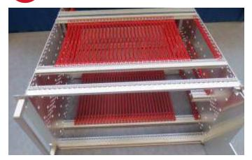
Customer needs a 6U subrack with recessed mounting front for cabling. All must be covered by a side hinged front panel. Guide rails for the PCB's must be assembled (assembly service). Mixed 3 and 6U boards inside the subrack.
