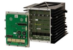
A conduction cooled chassis was selected. In order to achieve the required processing power the PICMG standard CompactPCI was chosen for the system architecture. A special solution was created to seal the chassis according to IP65, even with the thin side, bottom and top plates. The project was completed in cooperation with the system integrator EMCOMO.
