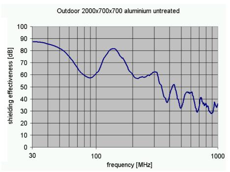
Typical shielding effectiveness, in the frequency range from 30 MHz to 1000 MHz. Calculated with the worst case of each examined side and smoothing of the resonance frequencies.
